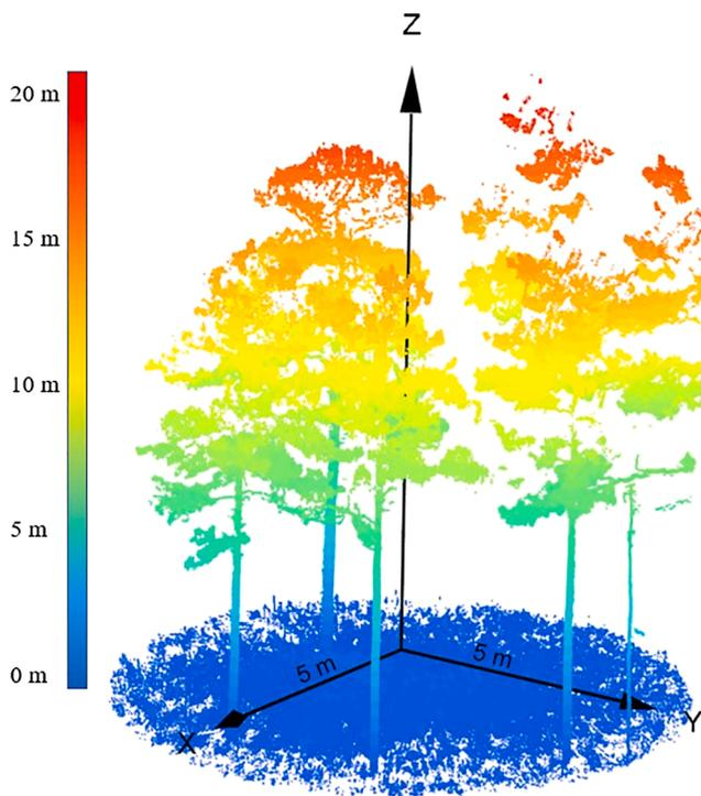
Fig. 2. An example of a clip from a Terrestrial LiDAR scan point cloud taken using the Leica BLK360. The color gradient shown represents the height (Z) of returns in meters.
